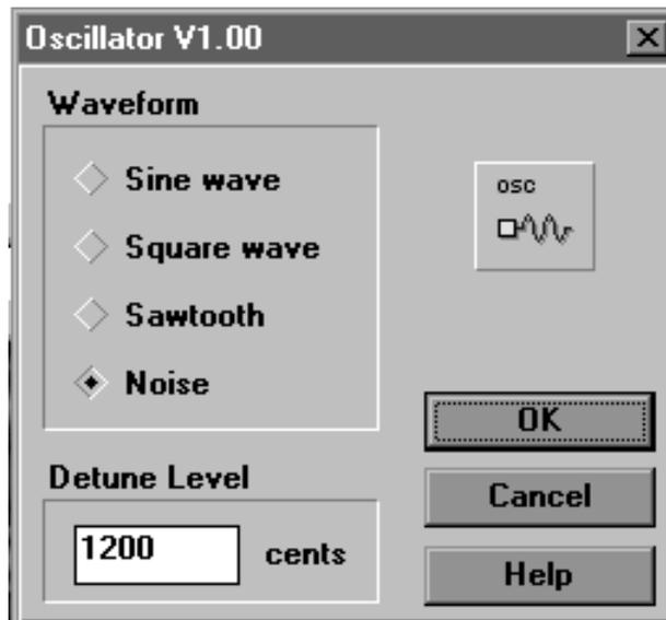
Figure 8.5 The dialogue box to set the parameters for an oscillator. Specific parameter settings for each module are specified via dialogue boxes which are accessed by double-clicking with the left mouse button over the modules
