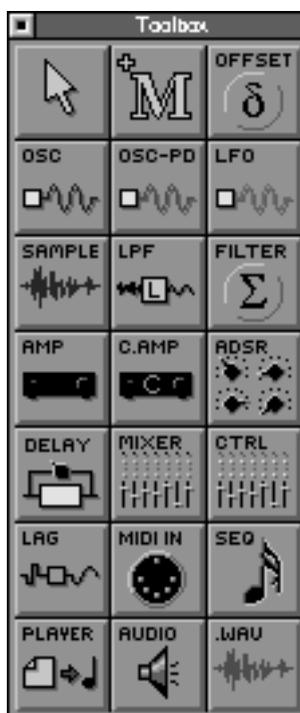
**Figure 8.3** Audio Architect provides a menu of synthesis modules that mimic the various components of an analog synthesiser
