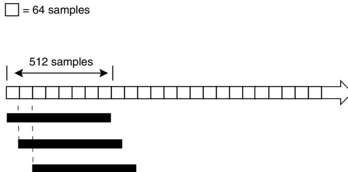
**Figure 3.12** In this case a window has 512 samples and the overlap factor is set to 64 samples ( $512/8 = 64$ )
